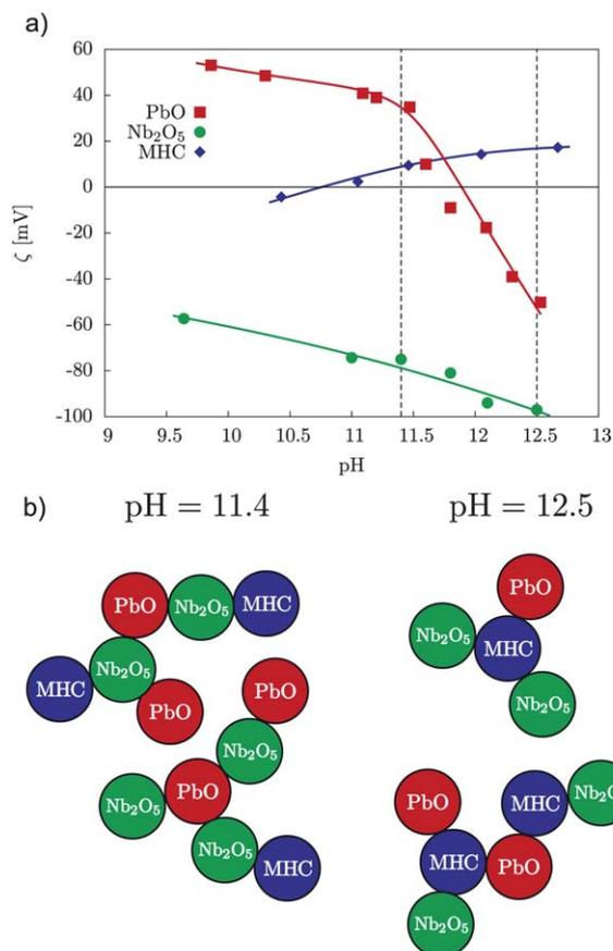
**Fig. 1** a) Measured zeta-potentials of PbO, Nb<sub>2</sub>O<sub>5</sub> and MHC particles as a function of the suspension pH. The two pH conditions considered in experiment and simulations are denoted by dashed lines. b) Schematic presentation of the predicted cluster formation in the suspensions with pH = 11.4 and pH = 12.5.
