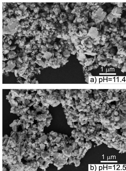
**Fig. 2** FE-SEM micrographs of the dried powder mixtures for a) pH 11.4 and b) pH 12.5 samples. In both samples sub-micrometre particles are observed, which is in agreement with the light scattering measurements.<sup>5</sup>
