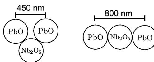
**Fig. 4** Schematic presentation of two PbO particles adsorbed on the Nb<sub>2</sub>O<sub>5</sub> particle. The closest distance between two PbO particles is at 450 nm (repulsive potential), left configuration, and the largest at 800 nm, right configuration.
